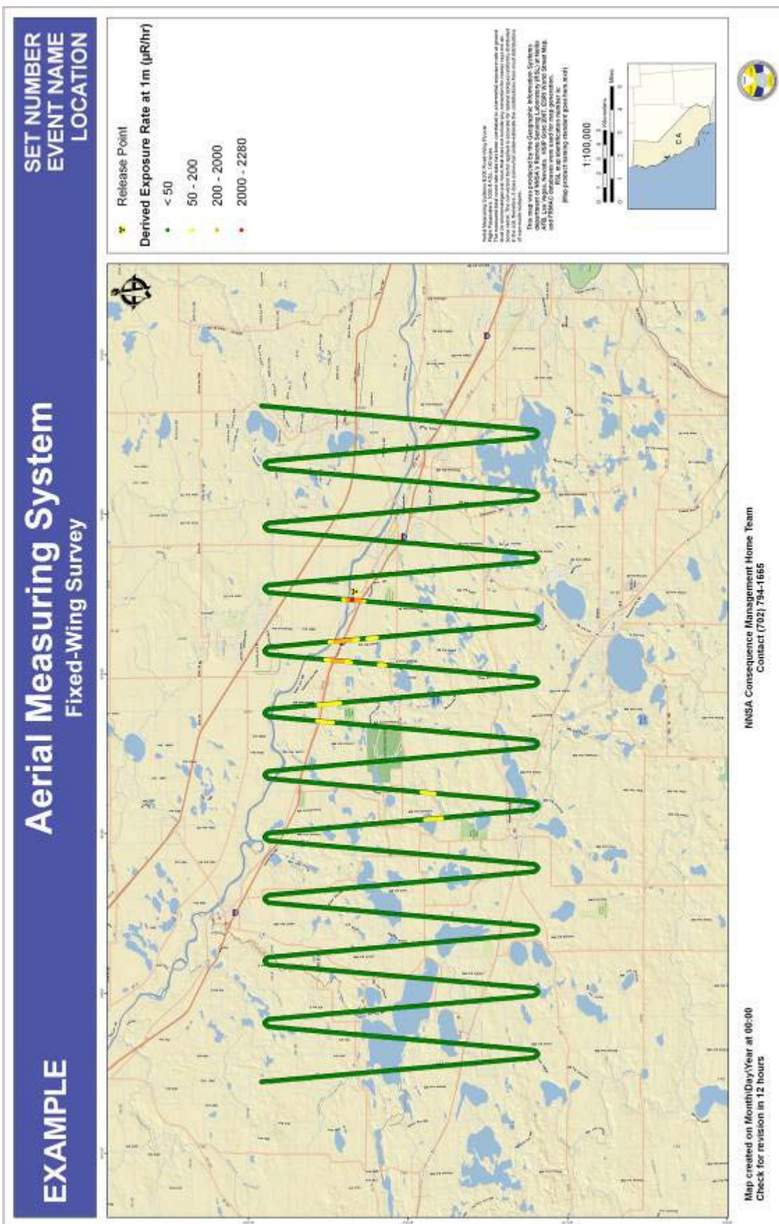
FIGURE C-1. SERPENTINE FLIGHT PATTERNS (EXPOSURE RATES)
